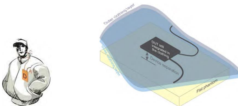
Figure 10– Test position for clothing-integrated wireless devices
