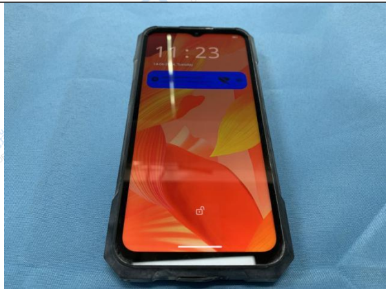
Fig.19 Power on inspection after test
