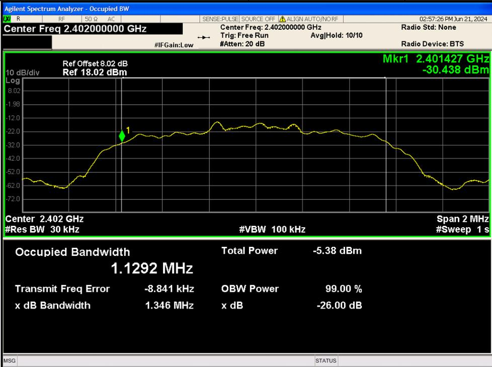
Modulation Type: Pi/4DQPSK      Test Channel: Highest Channel
