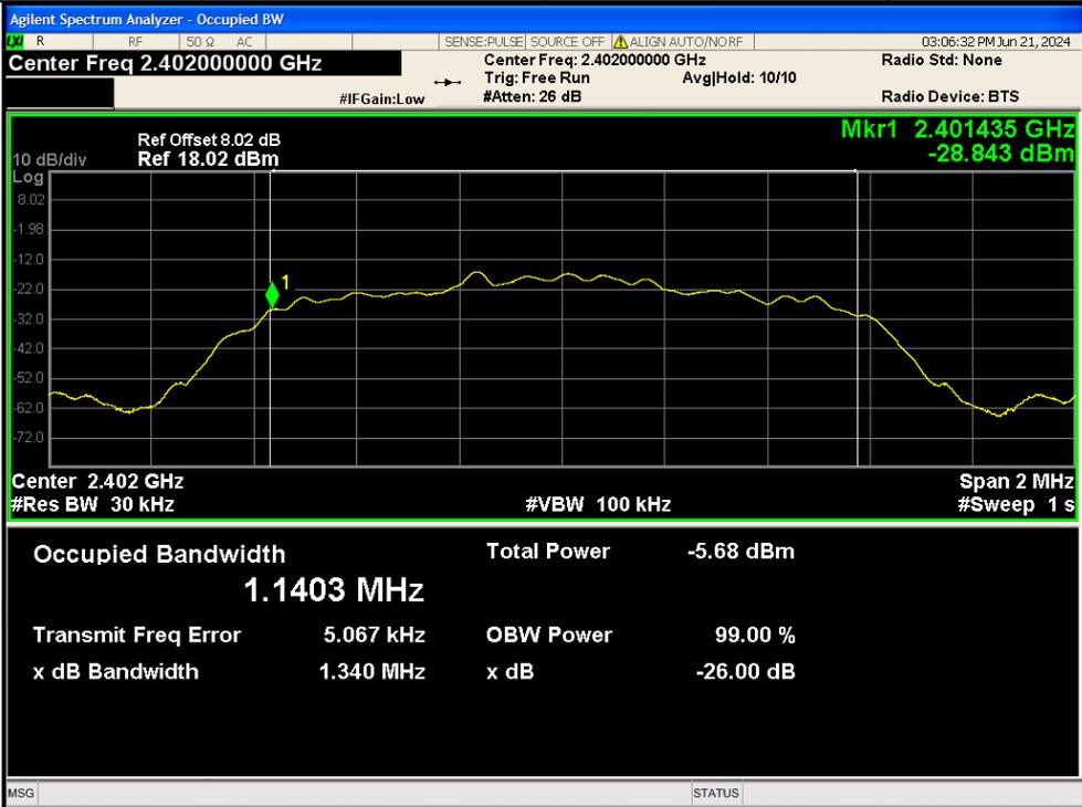
Modulation Type: 8DPSK Test Channel: Highest Channel
