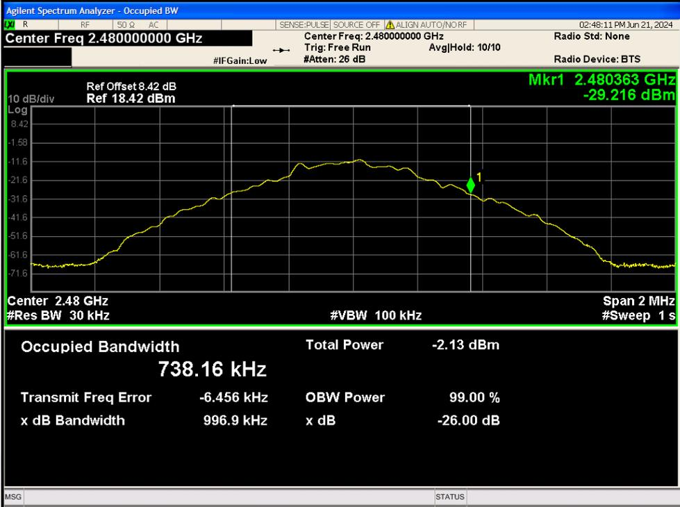
Modulation Type: Pi/4DQPSK      Test Channel: Lowest Channel
