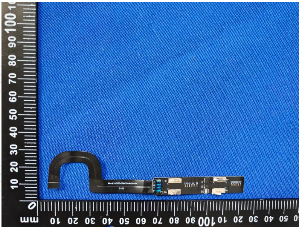
Picture 5. Front view of protection board 图片 5. 保护板前视图
