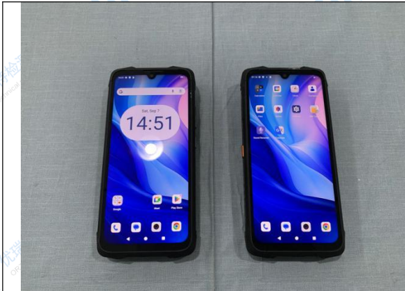
Fig.66 Power on inspection after test
